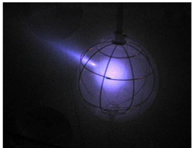
Photograph of an inertial electrostatic confinement fusion reactor operating in its "jet" mode in order to release a portion of the fusion plasma
